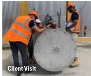
Factory Acceptance Testing of AWMA Modular Stoplogs
